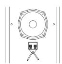
(4) If you use the sliders, you can mount the speaker cables to the terminal at this point. If you use the mounting points, it is easier to install the speaker first and mount the cable to the terminal after the speaker is mounted to the wall.
