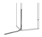
3 Run the speaker cable through the tube positioned at the rear of the cabinet to the terminal at the front baffle.
